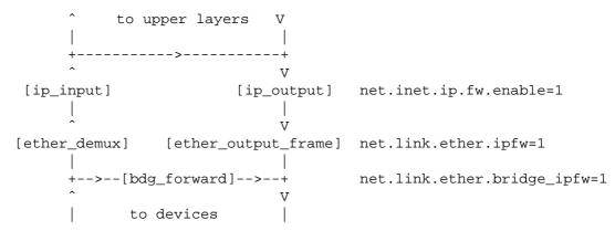
As can be noted from the above picture, the number of times the same packet goes through the firewall can vary between 0 and 4 depending on packet source and destination, and system configuration.
